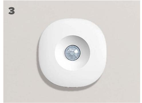
Resident health data is passively and privately collected via **1. a depth sensor** that uses infrared (IR) technology to take precise measurements that calculate movement, walking speed, gait, stride and TUG score; **2. a bed sensor** under the mattress to trend restlessness, bed occupancy, sleep quality, etc.; and **3. one or more motion sensors** to cover areas where the depth sensor would not cover.
